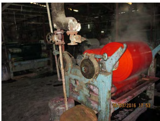
Caption: Cotton dyeing using jigger machines
